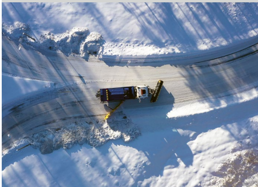
An Arctic Road Maintenance Truck with lateral plough, as used by Tapio Pahkakangas.
