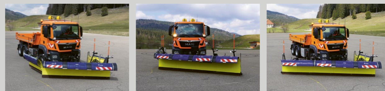
The Schmidt Tarron HP-2W high-performance snowplough can clear a width of up to 6.2 metres.
